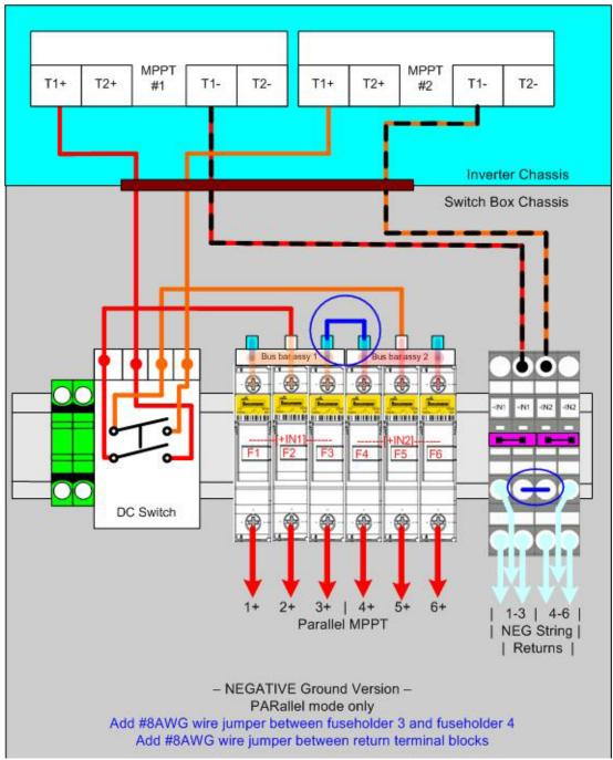
Figure 3.14b - Parallel mode-negative ground version *PVI-10/12-I-OUTD-S2-US/CAN--XXX With Fuse Holders*
