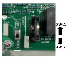
Figure 3.12 - Grid-Type configuration; 3W-Δ/4W-Y
