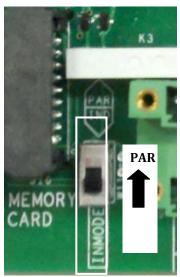
Figure 2.14a - Parallel Mode switch configuration
