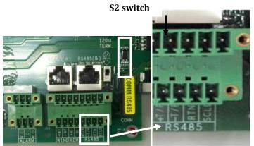
Figure 2.09 - Standard RS485 connection
