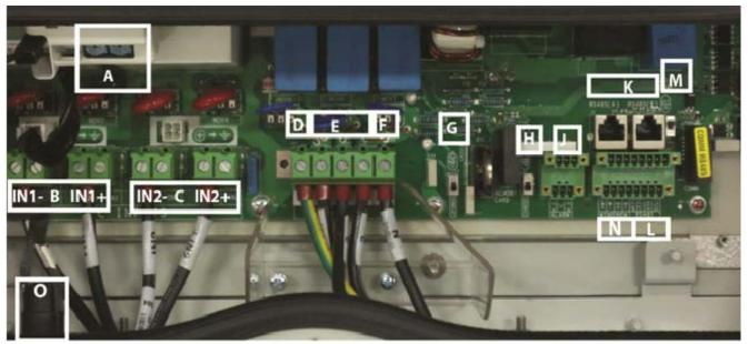
Figure 1.04 - Wiring Connection Details for PVI-10/12-I-OUTD-US/CAN-XXX
