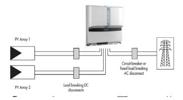
Figure 7.02 - Simplified Diagram of a Photovoltaic System
