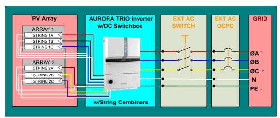
Figure 2.05 - Electrical Connection Diagram PVI-10.0-I-OUTD-S1-US/CAN-XXX-YY
