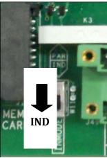
Figure 1.13 - INMODE switch set to IND mode
