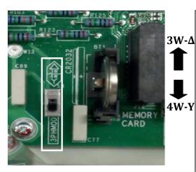
Figure 2.12 - Phase configuration 3W-Δ/4W-Y
