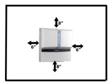
Figure 0.02 - Minimum Clearances around the AURORA Inverter
