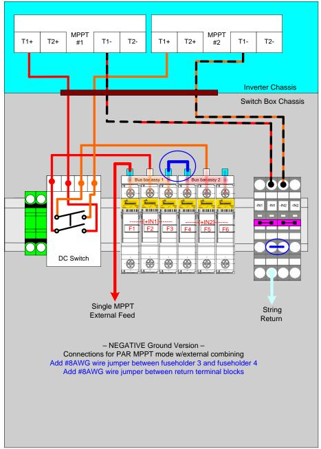
Figure 3.14d - External Combiner feed for Single/Parallel MPPT operation (Negative Ground Version)
