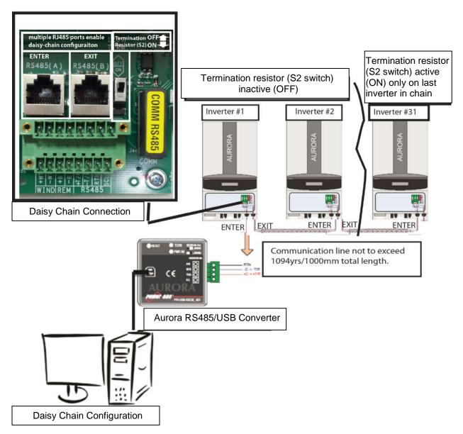
Figure 3.15 - Daisy Chain Connections and Configuration
