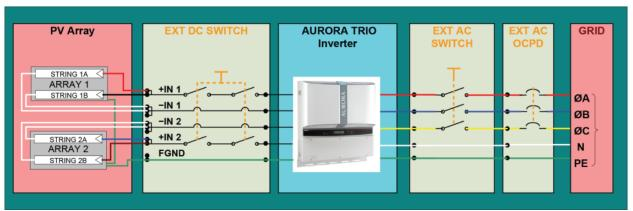
Figure 1.05 - Electrical Connection Diagram PVI-10/12-I-OUTD-US-XXX-NG
