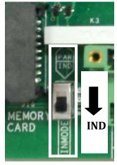
Figure 2.13 - INDependent mode switch configuration
