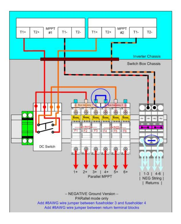
Figure 2.14b - Large switchbox with combiners showing jumpers (circled) required for Parallel MPPT Input Connection *PVI-10.0-I-OUTD-S1-US/CAN-XXX-YY*
