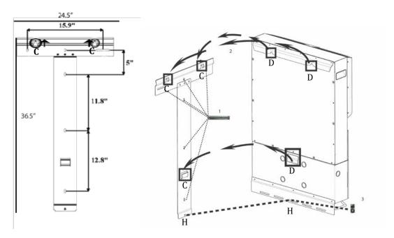
Figure 2.01 - Bracket and Mounting Details PVI-10.0-I-OUTD-S1-US/CAN-XXX-YY
