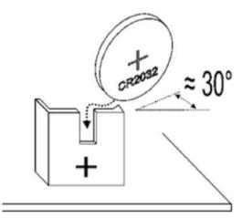
Figure 6.04 Lithium Battery Replacement
