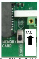
Figure 3.14a - Parallel Mode Configuration Switch
