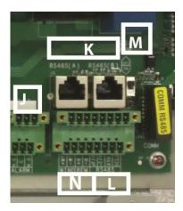
Figure 1.08 - Signal Configuration Connections PVI-10/12-I-OUTD-US/CAN-XXX-NG
