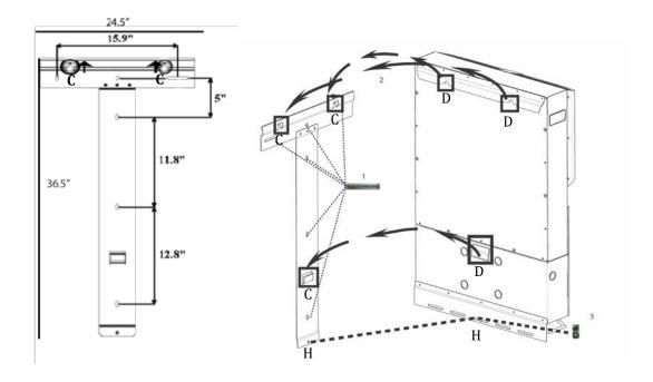
Figure 3.01 - Bracket and Mounting Details PVI-10/12-I-OUTD-S2-US/CAN-XXX
