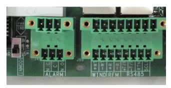
Figure 4.05 - Alarm contact terminal block
