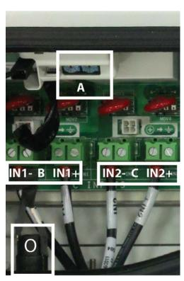
Figure 6.03 - GFD Fuse Location
