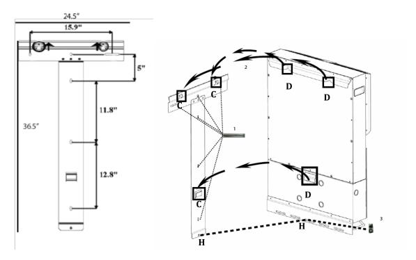
Figure 2.01 - Bracket and Mounting Details PVI-10.0-I-OUTD-S-US-XXX-YY
