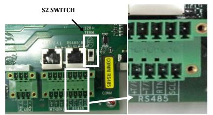
Figure 1.09 - Standard RS 485 Connection
