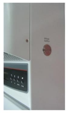
Figure 4.01- Inverter Stand-by Supply Button
