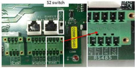
Figure 2.09 - Standard RS485 Connection
