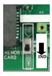
Figure 2.13 - Independent MPPT Configuration Switch
