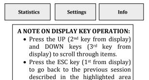
• Press ENTER (4th key from display) to open the selected submenu.
