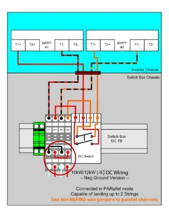
Figure 2.14b - Switchbox Jumpers for Parallel MPPT Input Connection PVI-10.0-I-OUTD-S-US-XXX-YY
