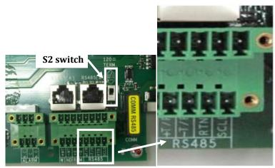
Figure 3.09 - Standard RS485 connection
