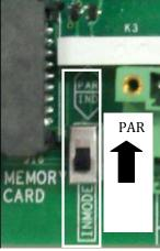
Figure 2.14a - Parallel MPPT Configuration Switch
