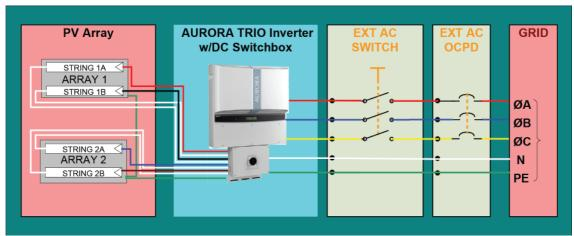
Figure 2.05 - Electrical Connection Diagram PVI-10/12-I-OUTD-S-US/CAN-XXX-NG
