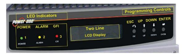
Figure 5:01- Location of the buttons and LEDs
