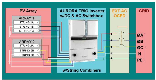
Figure 3.05 - Electrical Connection Diagram PVI-10/12-I-OUTD-S2-US/CAN--XXX With Fuse Holders
