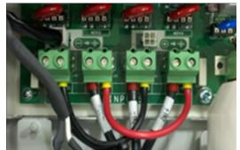
Figure 1.14b - Jumpers for Parallel MPPT Input Configuration PVI-10/12-I-OUTD-US/CAN-XXX-NG
